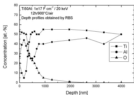
Fig. 2: Depth profiles of Ti, Al and O obtained by RBS (10<sup>17</sup> F cm<sup>-2</sup> and 12h/900°C/air).
