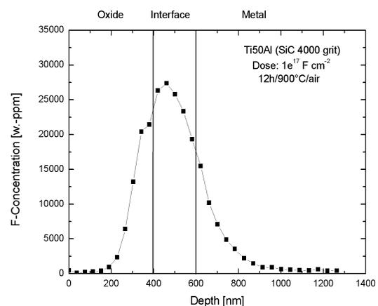
Fig. 1: F-Depth profile obtained by PIGE (10<sup>17</sup> F cm<sup>-2</sup> and 12h/900°C/air).
