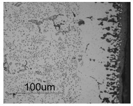
Microstructures of alloys after 500 cycles at 1100°C in  $H_2$  / CH<sub>4</sub> / H<sub>2</sub>O.
