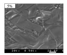
Figure 1: SEM Micrograph of the Surface of  $Si_3N_4/Y_2O_3+Al_2O_3$  Ceramics Containing 5 volume % CrB<sub>2</sub> After Oxidation at 1400°C for 10 Hours
