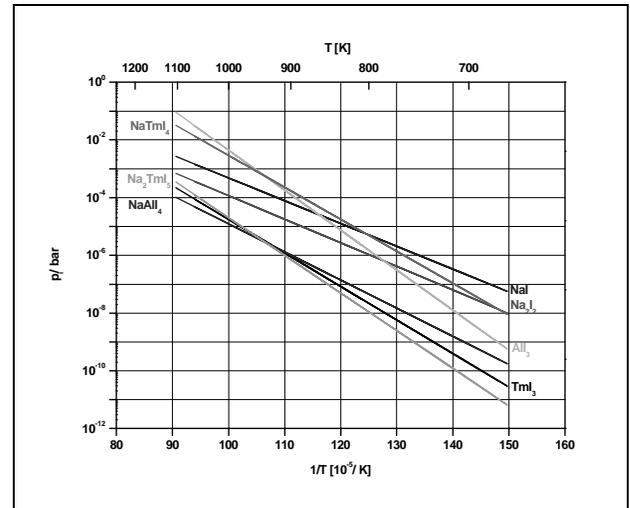
Fig. 2: Partial pressure over an equimolar mixture of  $\text{NaI} / \text{TmI}_3 / \text{Al}_2\text{O}_3$
