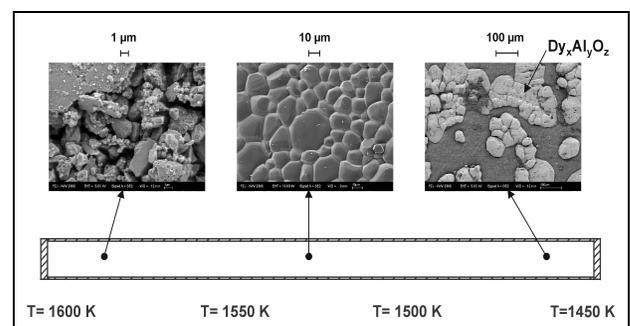
Fig. 3: SEM investigation of the PCA vessel after the annealing in a temperature gradient for 1000h
