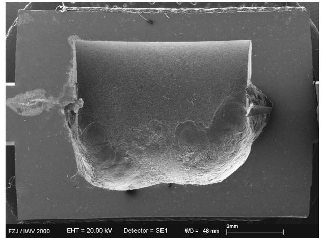
Fig. 1: Cross section of a PCA-discharge burner after 9000h of operation
