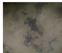
Fig. 1 POM image of Zn(acac)_2 at 87°C
