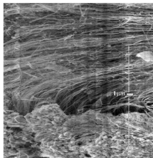
Fig.1 SEM image of straight ropes horizontally aligned bundles.
