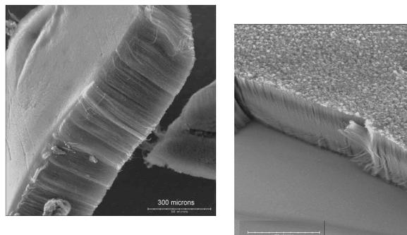
iron-rich sample (16.5 wt%) is obtained at 750  $^{\circ}\text{C}$ , and the iron-poor sample (2.6 wt %) is obtained at 850  $^{\circ}\text{C}$  which seems to be the cleanest according to SEM observations.
