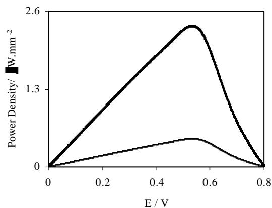
Figure 1. Dependence of the power output on the cell voltage with the cathode implanted near the skin of the grape (heavy line); and with the cathode implanted near the center of the grape (fine line).
