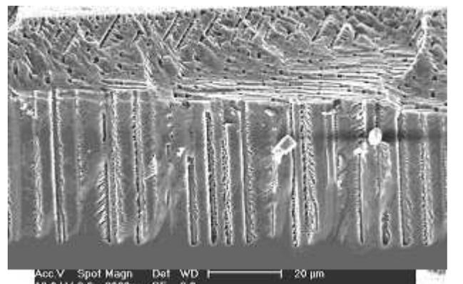
**Fig. 3:** Cross section (SEM) of (111) - oriented silicon etched in conducting salt containing organic electrolyte: In the upper part crystallographic pores have been formed at low voltages (1V). Increasing the potential to 3V, induces current line pores growing nearly perpendicular to the surface.
