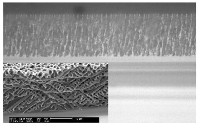
**Fig. 2:** Cross section of the wafer from Fig. 2 (optical microscope): Starting at the nucleation sites at the top of the (111) oriented wafer pores grow almost perpendicular into the wafer in contrast to the normally growing 113 pores on a (111) silicon substrate (see inset).
