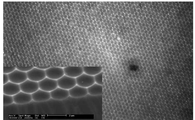
**Fig. 1:** Optical microscope image of the surface after etching a prestructured wafer – at all nucleation sites pores grew. Inset: SEM plain view (tilted) of unetched prestructuring mask.
