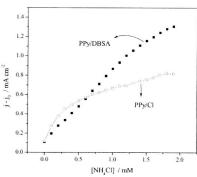
the polymeric film during the ammonia detection is affected by the dopant anion: small changes are observed by films doped with large anions, as it was followed by EQCM experiments. Raman spectroscopy revealed that no drastic changes occur in the polymeric chain during the detection, except the diminution of the band at 1250 cm<sup>-1</sup>.
