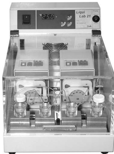
Figure 3: LiquiLab with 4 measurement chambers with pumps for pulse-free sample transport and minimized sample volume
