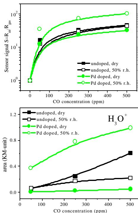
Fig 2. top: Sensor signal of Pd and undoped sensor in dry and humid air. Bottom: Band analysis for hydrated proton species in dry and humid air.
