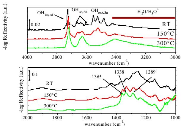
Fig 1: DRIFT spectra at different temperatures. Top: OH/H<sub>2</sub>O range, bottom: carbonate range
