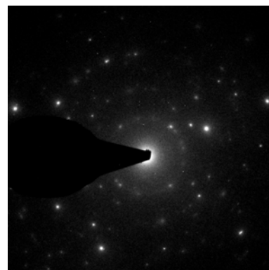
Figure 2. SAED elicits nanopolycrystalline ring structure.
