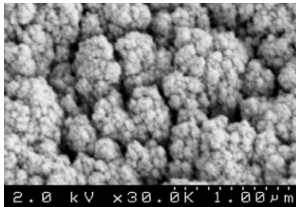
Fig. 3. SEM image of a Cu-Zn-O porous membrane, in plan view, that was reactively sputter deposited for use in catalytic hydrocarbon reformation.
