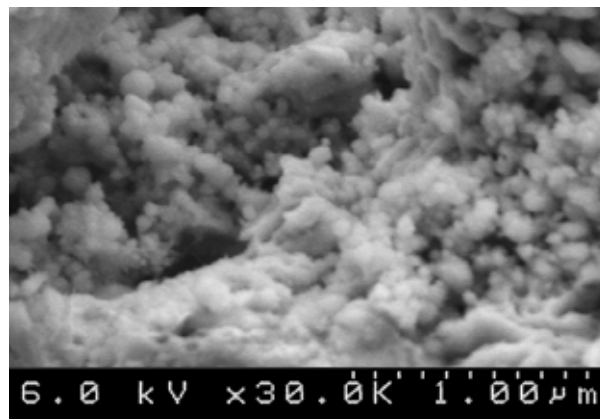
Fig. 2. SEM image of a porous, nanostructured Cu membrane viewed in cross-section that was sputter deposited at high temperature and gas pressure.
