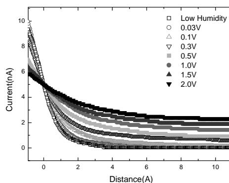
Fig. 2. Tunneling current versus distance characteristic measured on an Au(111) surface with a Gold tip at relative humidity 95% and tip bias voltage 0.03V, 0.1V, 0.3V, 0.5V, 1.0V, 1.5V, 2.0V, Low humidity.
