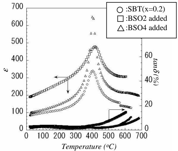
Fig.2 Dielectric constant,  $\epsilon$ , and  $\tan\delta$  at 1MHz dependence of temperature for SBT( $x=0.2$ ) and BSO added samples.
