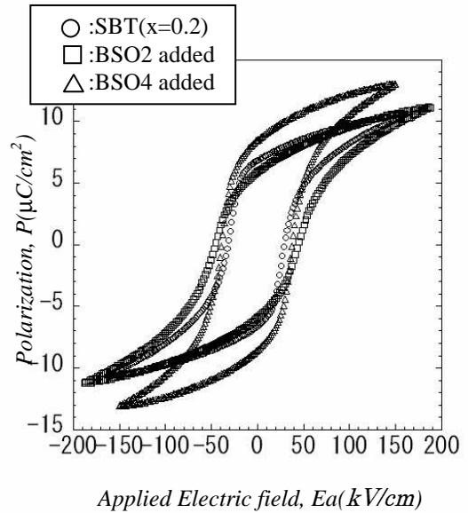
Fig.1 P-E hysteresis loops of SBT( $x=0.2$ ) and BSO added samples at 10Hz.
