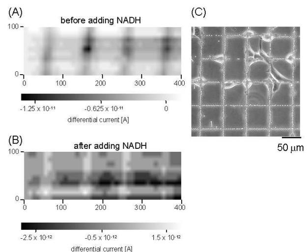
Figure 3. SECM image of the enzyme activity of diaphorase immobilized on microparticles without (A) and with 5 mM NADH (B). Microscopic photograph of cultured MCF-7 cells on patterned particles (C).
