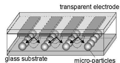
Figure 1. Principle of the dielectrophoretic patterning of microparticles.
