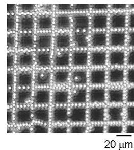
Figure 2. Microscopic photographs of patterned  $\phi$  3  $\mu\text{m}$  amino-derivative particles in Grid formations.
