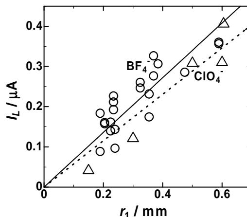
Fig.2 Proportionality of the limiting current with radii of contacting circles of the PDS droplets when the aqueous solution included 0.05 M NaBF<sub>4</sub> (circles) and 0.050 M NaClO<sub>4</sub>. (triangles). The oil phase contained 10 mM ferrocene. Voltammograms were obtained at 10 mV s<sup>-1</sup>.
