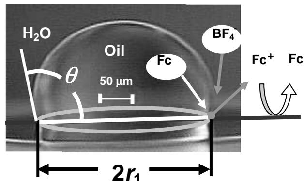
Fig.1 Photograph of the ferrocene-included polydimethylsiloxane droplet on the glassy carbon electrode in 0.1 M NaBF<sub>4</sub> aqueous solution. The arrows are the predicted transport of ferrocene, ferricenium ion and BF<sub>4</sub><sup>-</sup>.
