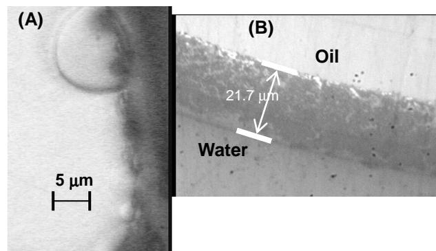
Fig.3 Photographs of the PDS droplet on the electrode in 0.05 M KCl aqueous solution. (A) 10 minutes after applying 0.8 V, (B) 30 minutes after applying 0.8 V, the droplet was rinsed with water several times in order to remove water-dissolved salt before being mounted on the microscope. Then the droplet was dried on the electrode 60 min after the irradiation of the light beam of the microscope.
