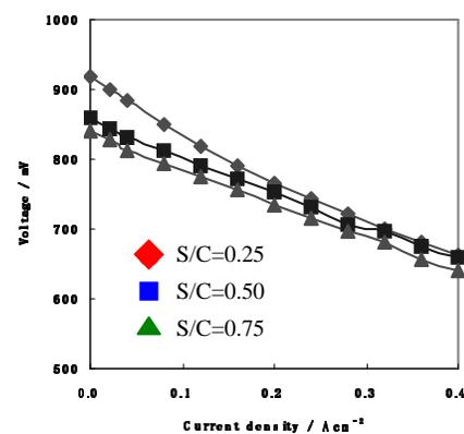
Fig.3: I-V characteristics of YSZ-supported cells for simulated biogas at 1000°C.
