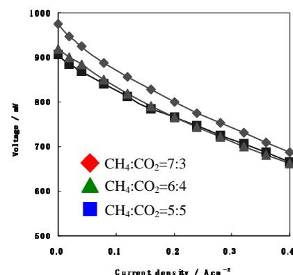
Fig.4: I-V characteristics of YSZ-supported cells for simulated biogas at 1000°C.
