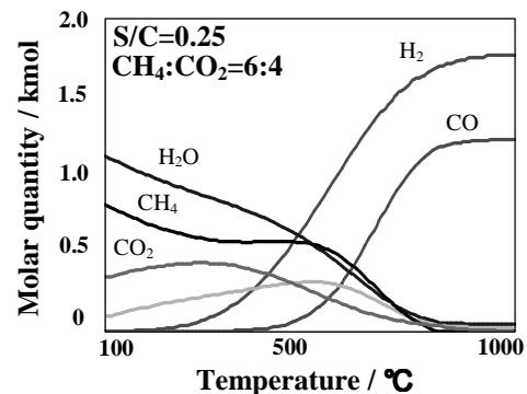
Fig.2: Equilibrium products from biogas with the steam-to-carbon ratio of 0.25.
