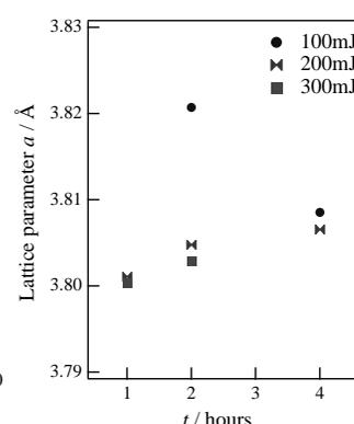
Fig.3 Deposition time dependence of lattice parameters for LSC films.
