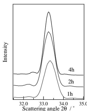
Fig.2 X-ray diffraction patterns for LSC film deposited for 1,2 and 4h.
