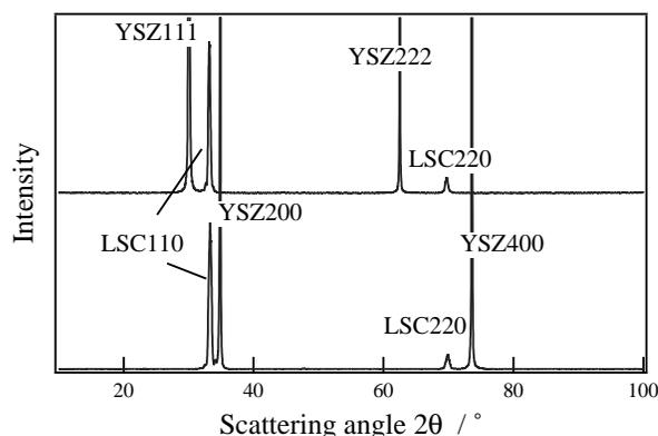
Fig.1 X-ray diffraction patterns for LSC films deposited on YSZ(100), (111).
