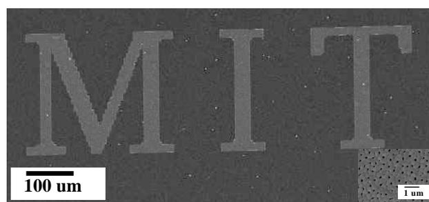
Fig. 3 Formation of porous alumina on patterned substrates. Pores form only on the patterned letters "MIT". The figure on the bottom right shows an inset of the pores
