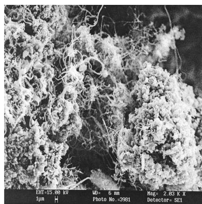
Fig.2 SEM of the electrosynthesized gadolinium boride
