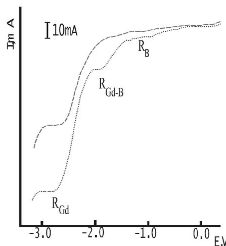
Figure 1. Voltammograms of the molten systems: a –  $NaCl-KCl-NaF(10wt\%)-GdF_3(1.6 \cdot 10^{-4} \text{ mol} \cdot \text{cm}^{-3})$ ; b –  $NaCl-KCl-NaF(10wt\%)-GdF_3-KBF_4$  (molar  $B/Gd=0.25$ ); Mo-working electrode, GC-counter electrode, GC-reference electrode; 1023 K,  $v=0.1 \text{ V} \cdot \text{s}^{-1}$
