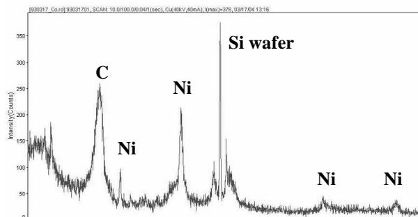
Fig. 3 XRD pattern of the Ni/CNFs nanofibers array.
