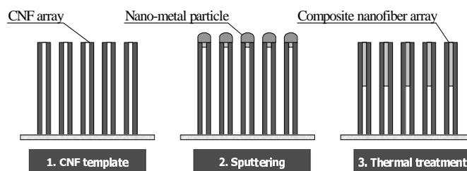
Fig. 1 Flowchart of the preparation of the composite nanofibers array.
