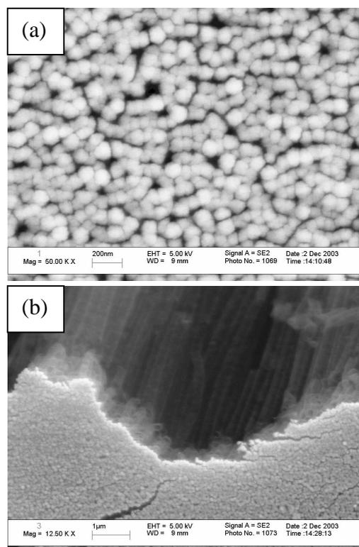
Fig. 2 SEM images of the Ni/CNFs nanofibers array.
