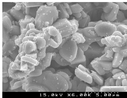
Fig. 1. SEM image of powders synthesized at 800 °C
