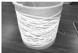
Figure 1. A spool of green \text{La}_{0.55}\text{Li}_{0.35}\text{TiO}_3 fiber with a diameter of 15 \mu\text{m}
