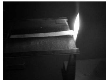
Figure 1. Sequence of flame test of conventional electrolyte with flame retardant.
