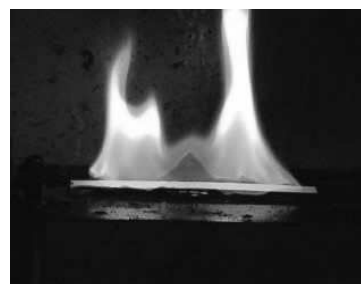
Figure 1. Sequence of flame test of conventional electrolyte with flame retardant.
