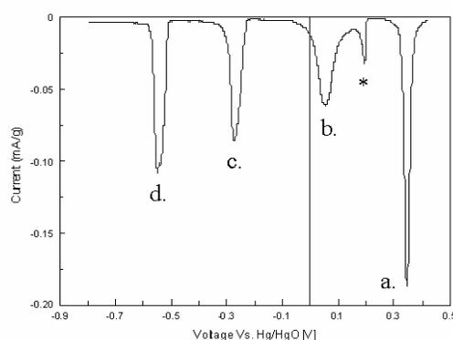
Figure 1: Linear sweep voltammogram of  $\text{AgCuO}_2$ , collected using sweep rate = 0.01 mV/sec. Four major discharge processes are observed at a. +0.35 V, b. +0.06 V, c. -0.28 V and d. -0.56 V. Discharge process at +0.18 V, denoted \*, corresponds to  $\text{Ag}_2\text{O}$  impurity. Voltages reported with respect to Hg/HgO reference electrode.
