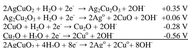
is proposed based upon analysis of ex-situ x-ray powder diffraction patterns of the discharge products.
