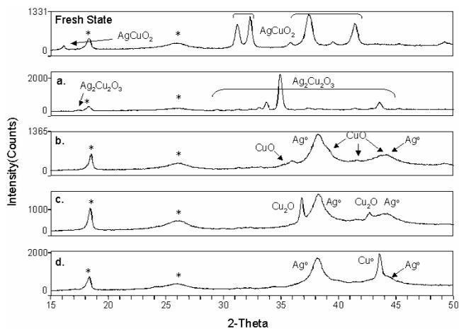
Figure 2: Ex-situ x-ray powder diffraction patterns of  $\text{AgCuO}_2$  cathode mixtures, corresponding to the discharge products from discharge processes a., b., c. and d. shown in Figure 1. Teflonized acetylene black denoted with \*.
