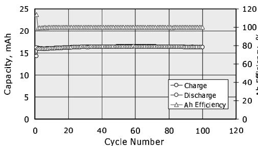
**Fig. 2** Cycling result of graphite/ $\text{Li}_{1+x}(\text{Ni}_{1/3}\text{Co}_{1/3}\text{Mn}_{1/3})\text{O}_2$  cell at 1C rate and 25°C.
