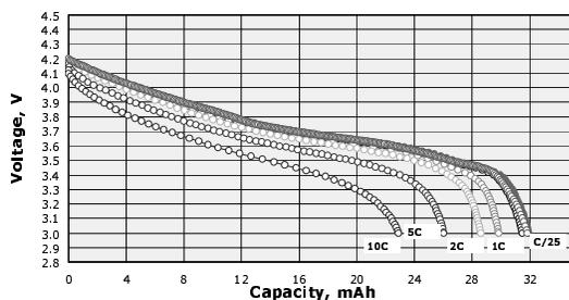
**Fig.1** Discharge curve of graphite /  $\text{Li}_{1+x}(\text{Ni}_{1/3}\text{Co}_{1/3}\text{Mn}_{1/3})\text{O}_2$  cell at room temperature.
