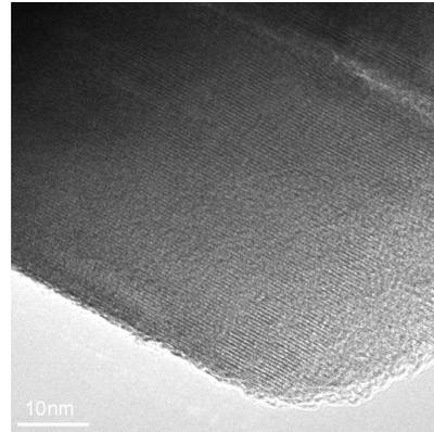
**Fig.3** TEM image of  $\text{Li}_{1+x}(\text{Ni}_{1/3}\text{Co}_{1/3}\text{Mn}_{1/3})\text{O}_2$  electrode after cycling.
