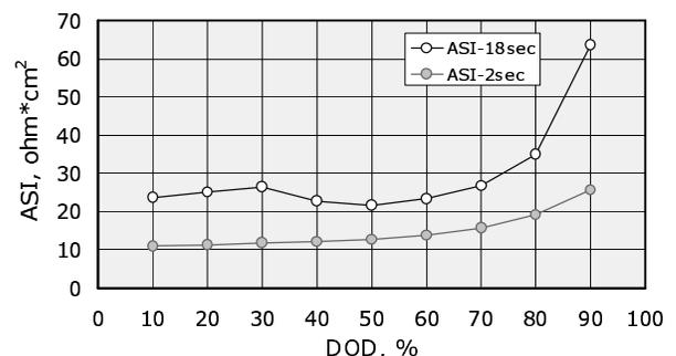
**Fig.4** ASI of graphite/ $\text{Li}_{1+x}(\text{Ni}_{1/3}\text{Co}_{1/3}\text{Mn}_{1/3})\text{O}_2$  cell during hybrid pulse power characteristics test.
