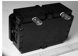
Fig. 1. 40W DMFC stack with external manifold type and Voltage-current characteristics change under changing temperature
