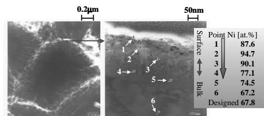
Figure 3 TEM images for Mm<sub>0.96</sub>Mg<sub>0.04</sub>Ni<sub>4.2</sub>Co<sub>0.3</sub>Mn<sub>0.4</sub>Al<sub>0.3</sub> alloy with B/A=5.2
