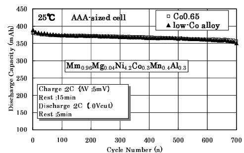
Figure 4 Comparison of cycle property in AAA-sized battery
