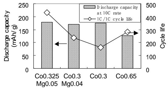
Figure 1 Comparison of discharge capacity and cycle life.
