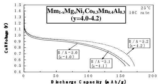
Figure 2 Discharge curves at 10C rate
