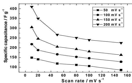
Fig. 1. SC of MnO<sub>2</sub>/SS electrodes calculated from CV against the scan rate. MnO<sub>2</sub> was prepared by potentiodynamic method at various scan rates (indicated in the inset) to a mass of 0.2 mg cm<sup>-2</sup>.
