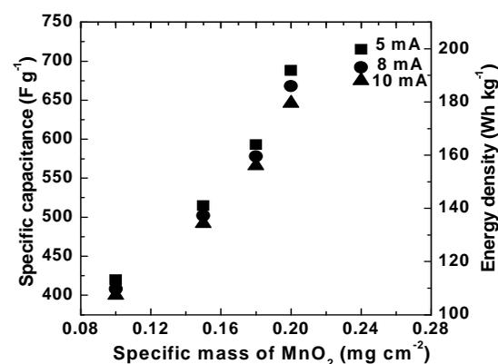
Fig. 2. SC and energy density of PANI-MnO<sub>2</sub> electrodes (at various discharge current densities) with various specific masses of MnO<sub>2</sub>. The specific mass of PANI was kept constant at 4 mg cm<sup>-2</sup>.
