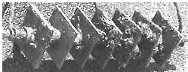
c: Immersed in open sea for 125 days
