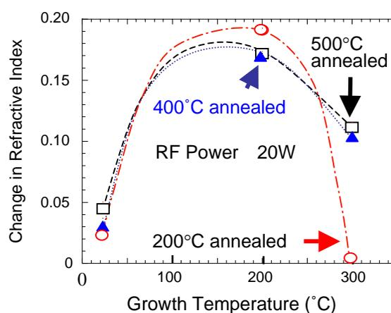
Fig. 2. Growth temperature dependence of the refractive-index change.
