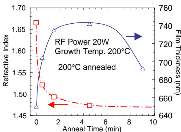
Fig. 1. Refractive index and film thickness versus anneal time for the sample grown at 200°C.
