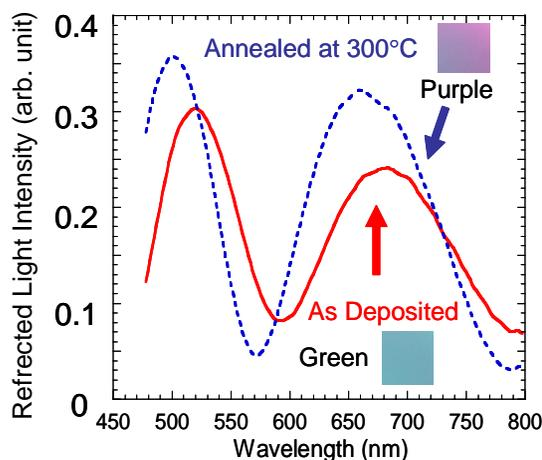
Fig. 4. Interference color change by the annealing. Growth temperature=300°C, initial thickness=610 nm, anneal temp=300°C, and anneal time=90 min.
