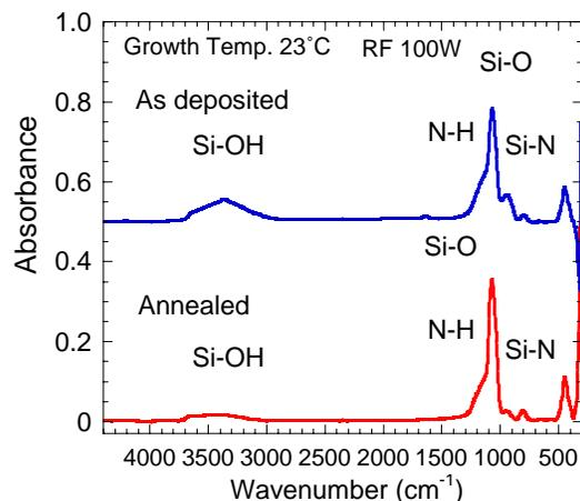
Fig. 3. FT-IR spectra of the as deposited and annealed (400°C, 30min) films.
