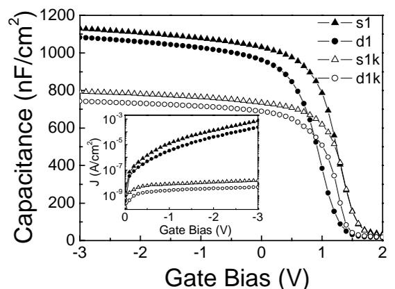
Fig. 2. The capacitance and leakage current density of MOS capacitors as a function of the gate bias.
