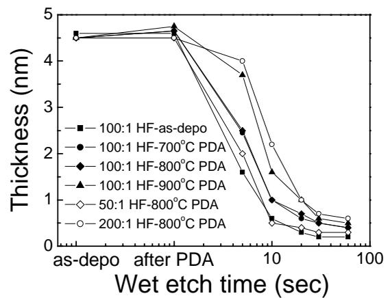
Fig. 1. The gate oxide thickness distribution of Al<sub>2</sub>O<sub>3</sub> films with the diluted HF concentration. The etch rate increased with a higher HF concentration and lower PDA temperature.
