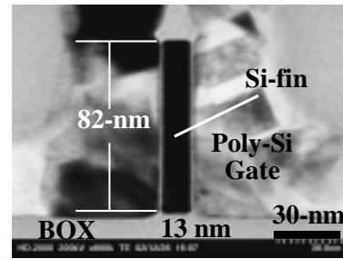
Fig. 1. Cross-sectional STEM image of the fabricated FinFET with an ideal rectangular channel shape.
