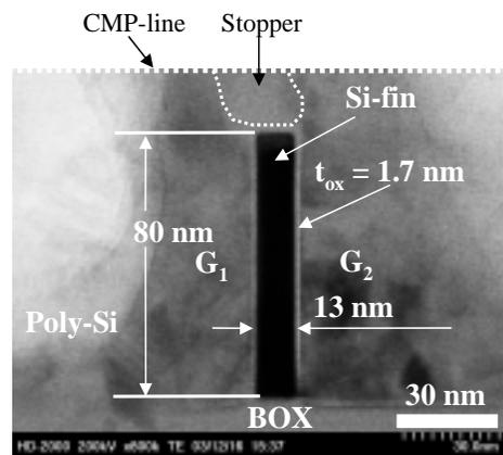
Fig. 3. Cross-sectional STEM image of the fabricated 4T-FinFET with a 13-nm thick Si-fin channel.
