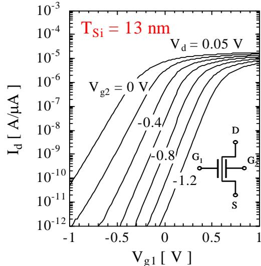
Fig. 4.  $I_d$ - $V_{g1}$  characteristics as a function of  $V_{g2}$  for the 4T-FinFET with 13-nm thick Si-fin channel.
