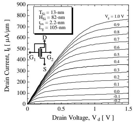
Fig. 2.  $I_d$ - $V_g$  characteristics of the fabricated FinFET with 13-nm Si-fin thickness and 105 nm gate length.
