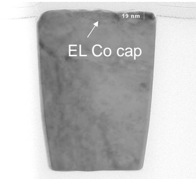
Figure 1. TEM cross-section of ALD TaN barrier and EL Co Cap layer
