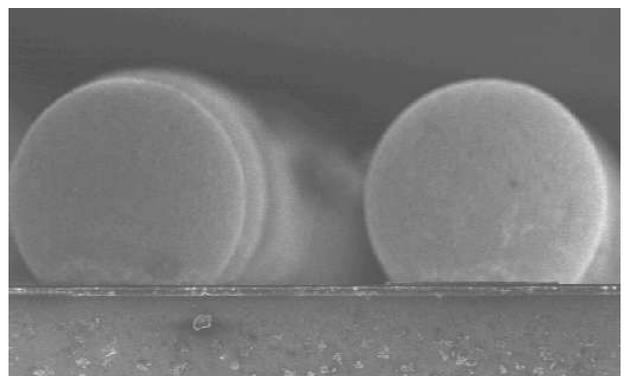
Figure 4. SEM photo of Sn bumps after reflow
