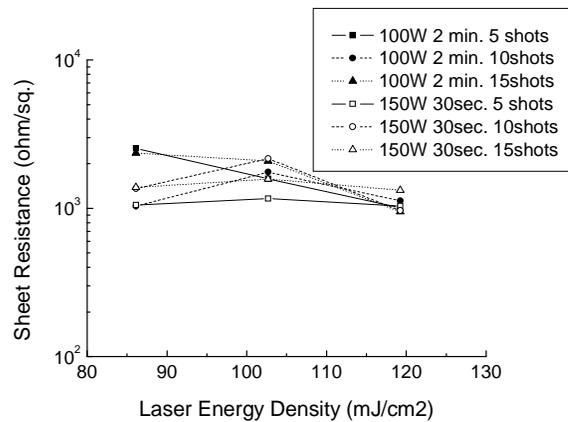
Fig. 2. Change in sheet resistance at two different levels of RF power for generating dopant ions.
