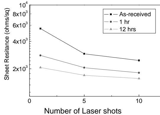
Fig. 1. Change in sheet resistance with additional thermal annealing at  $180^\circ\text{C}$  after the laser activation
