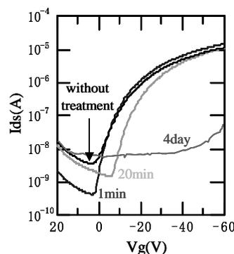
**Fig.2** Transfer characteristics. The channel length  $L$  is  $2000 \mu\text{m}$  and the channel width  $W$  is  $400 \mu\text{m}$  ( $V_{ds} = -20\text{V}$ ). The field effect mobility of TFT with ODT treatment for 1 min is  $0.24\text{cm}^2/\text{Vs}$ .
