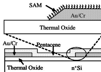
**Fig.1** Schematic TFT cross section.
