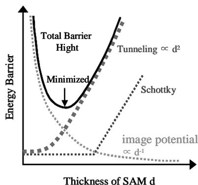
**Fig.3** Model of energy barrier at the interface between the electrode and semiconductor.
