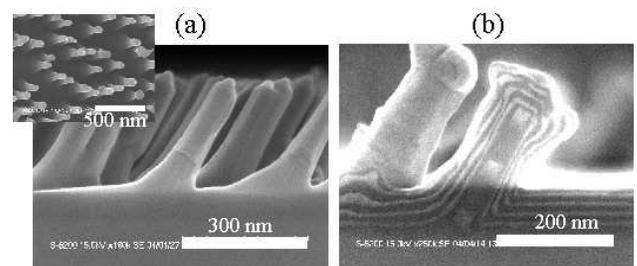
Fig. 2. SEM images of 3D nano-heterostructure cross sections. (a) AlGaAs buried structures (inset is top view) and (b) repeated GaAs/AlAs buried structures.
