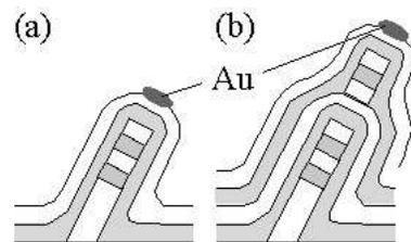
Fig. 1. Illustrations of 3D nano-heterostructure cross sections. (a) One process and (b) two processes of VLS and MOVPE growth modes.
