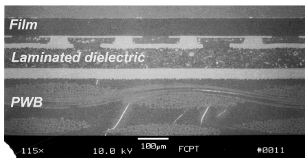
Figure 2 Transient liquid bonding formed between a flexible substrate and a rigid organic substrate.
