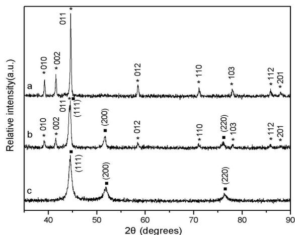
**Fig 1** XRD pattern of Ni synthesized in ethylenediamine at different temperature. (a)200°C,(b)250°C,(c)300°C.(\*)hcp phase nickel;(■) fcc phase nickel.Peaks represent fcc phase nickel (marked in parentheses)
