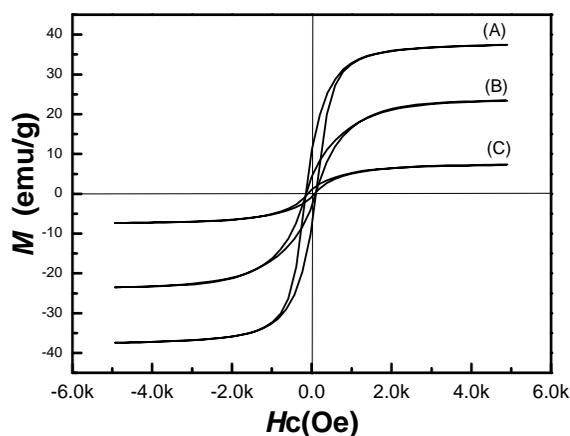
**Fig 3** Hysteresis loops of different crystal phase Ni at room temperature. (A)fcc, (B)fcc and hcp, (C)hcp
