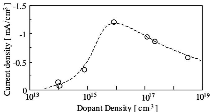
Figure 3. Plots of Reduction peak current density vs. dopant density of n-type Si.
