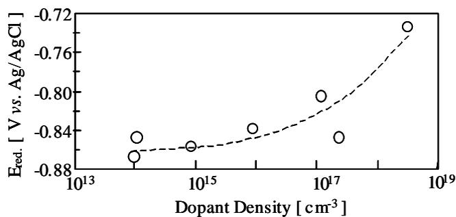
Figure 2. Dependence of reduction voltage on dopant density in n-type Si electrode.
