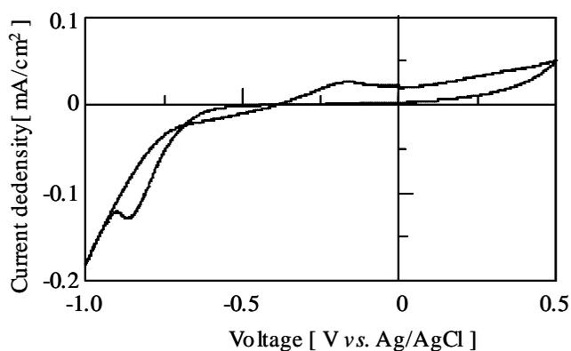
Figure 1. Cyclic Voltammogram carried out at Ni plating bath and Si electrode. The dopant density in Si is  $9.9 \times 10^{13} \text{ cm}^{-3}$ , P.
