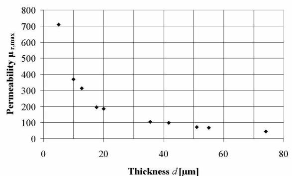
Fig. 2: Relative permeability  $\mu_{r,\text{max}}$  of NiFe 81/19 dependent on layer thickness  $d$
