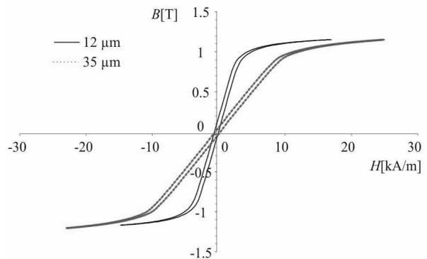
Fig. 1:  $BH$ -loops of 12 $\mu\text{m}$  and 35 $\mu\text{m}$  electroplated NiFe 81/19 layer
