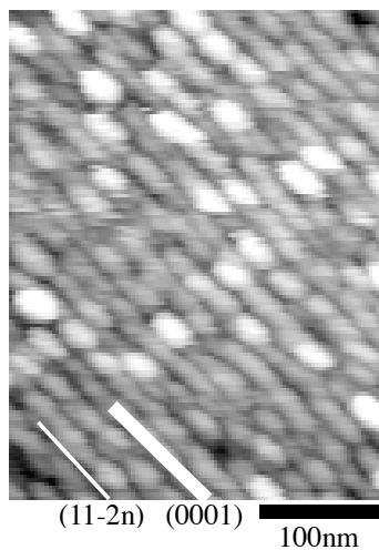
Fig. 3. AFM image of GaN growth on SiC by the nitridation of Ga at the time (b) in Fig. 1. GaN quantum wires are aligned along [1-100].
