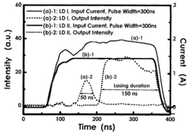
Fig. 2. Lasing duration characteristics of (a) LD I and (b) LD II. Both LDs were measured under a pulse width of 300 ns at room temperature.
