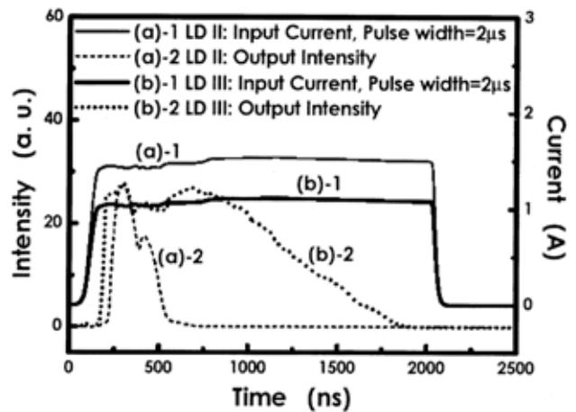
Fig. 3. Lasing duration characteristics of the (a) LD II and (b) LD III. Both LDs were measured under pulse width of 2 μs at room temperature.
