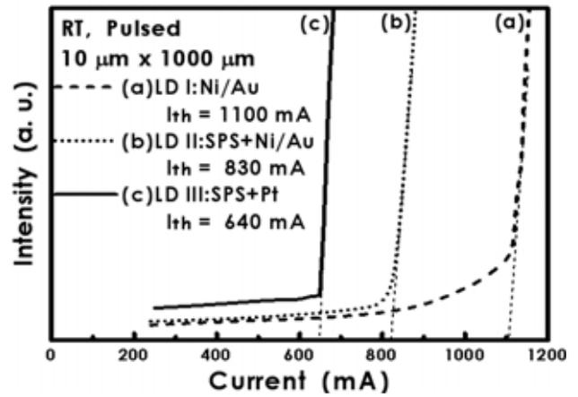
Fig. 1. Room-temperature L-I characteristics of the (a) LD I, (b) LD II, and (c) LD III.
