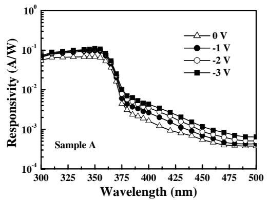
Figure 2 (a) Spectral responsivity of sample A.
