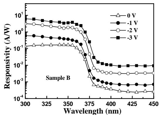
Figure 2 (b) Spectral responsivity of sample B.
