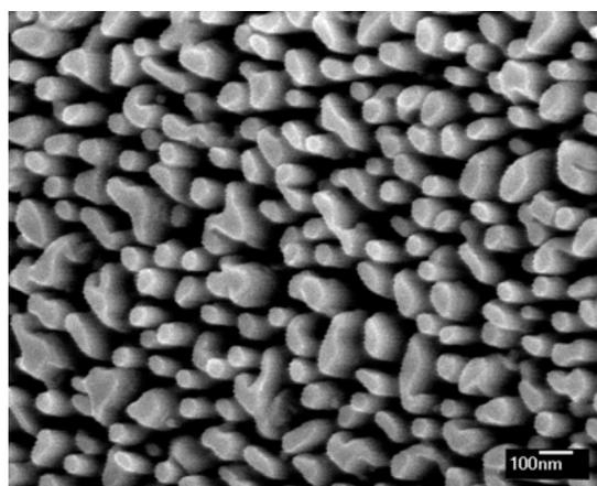
Fig. 2. High magnification top view of the InN nanocolumns.
