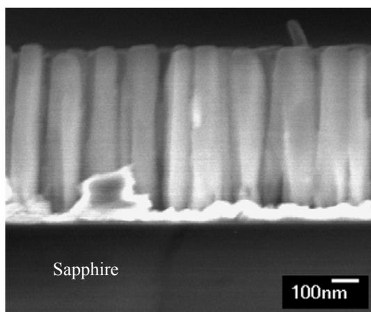
Fig. 3. Cross-sectional SEM image of the InN nanocolumns.
