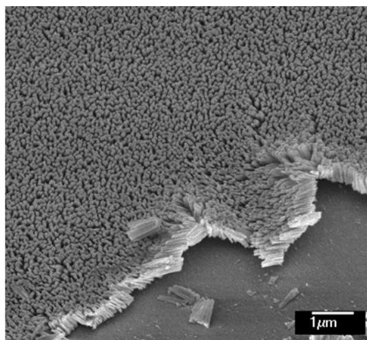
Fig. 1. SEM image of the InN nanocolumns grown on (0001) sapphire.
