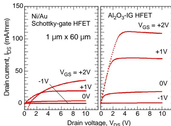
Fig.2 Drain I-V characteristics of the Ni/Au Schottky-gate and Al<sub>2</sub>O<sub>3</sub>-gate AlGaIn/GaN HFETs with the AlGaIn thickness of 7 nm.
