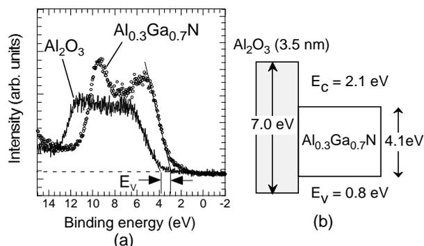
Fig.1 (a) XPS valence band spectra of the AlGaIn surface before and after the passivation and (b) band alignment at the Al<sub>2</sub>O<sub>3</sub>/AlGaIn interface.
