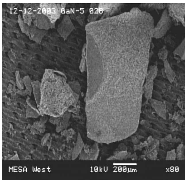
Figure 1 Scanning electron microscopy image of one of the crystals formed during molten salt electrolytic growth of GaN.
