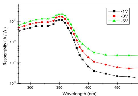
Fig. 3. Spectra responses of the typical Si-implanted planar p-n<sup>-</sup>-n<sup>+</sup> GaN photodetectors with reverse bias of 1, 3 and 5V.
