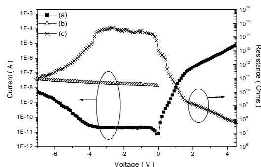
Fig.2. Logarithmic current-voltage characteristics of typical Si-implanted p-n<sup>-</sup>-n<sup>+</sup> GaN photodetectors. (a) dark current. (b) photocurrent illuminated at 350nm with a optical power of 12μW. (c) dynamic resistance  $R_d = (dI/dV)^{-1}$  derived from dark current.
